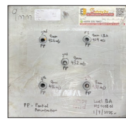
Safety2u Test Standard for Bulletproof Panel @ Door 7.62mm - NIJ STD 0108.01 (111)
